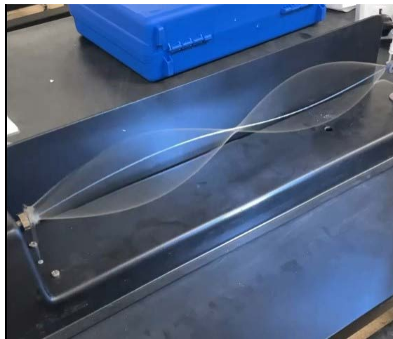
Figure 7.1: A student performing Melde's experiment ( n = 2 ).
