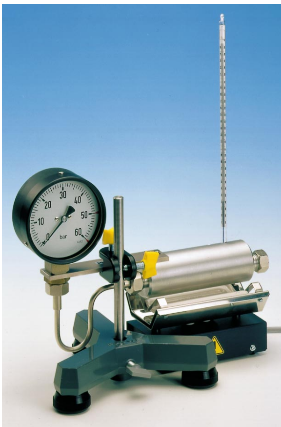
Fig. 1: Experimental set-up for measuring vapour pressure as a function of temperature.
