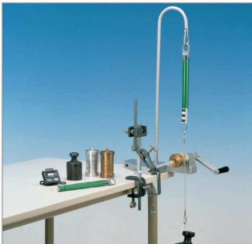
Fig. 1: Experimental set-up: Mechanical equivalent of heat.
