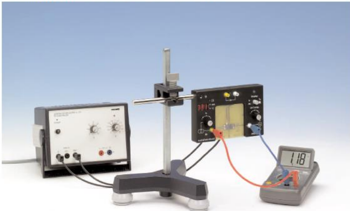
Fig.1: Experimental set-up for the determination of the band gap of germanium
