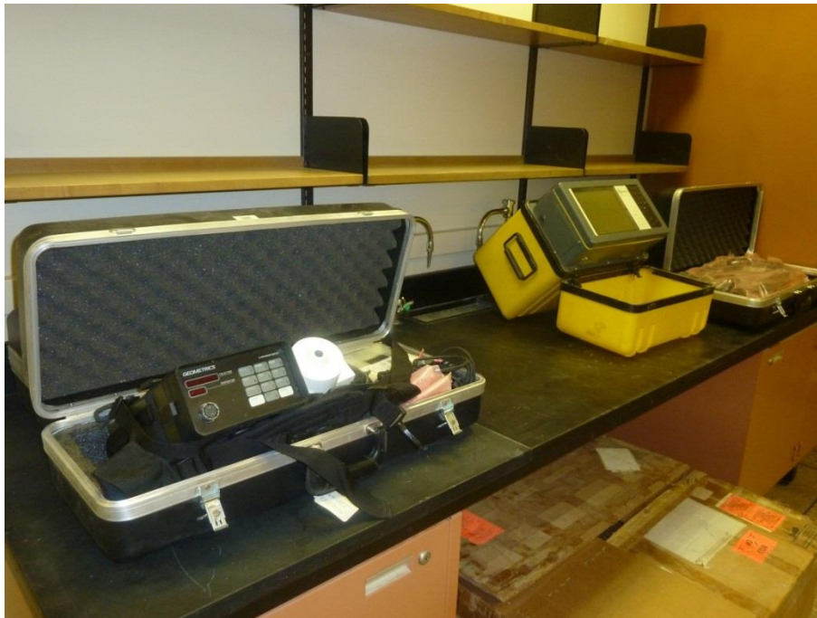
Magnetometers and seismograph unit
