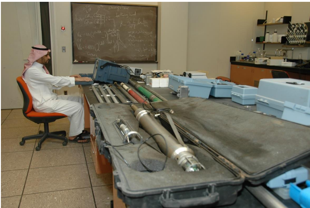
Borehole logging and Video Imaging Systems
