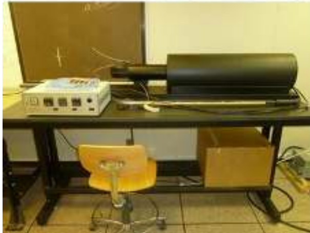
Rock magnetism unit (AF and Thermal demagnetization units, Spinner magnetometer)
