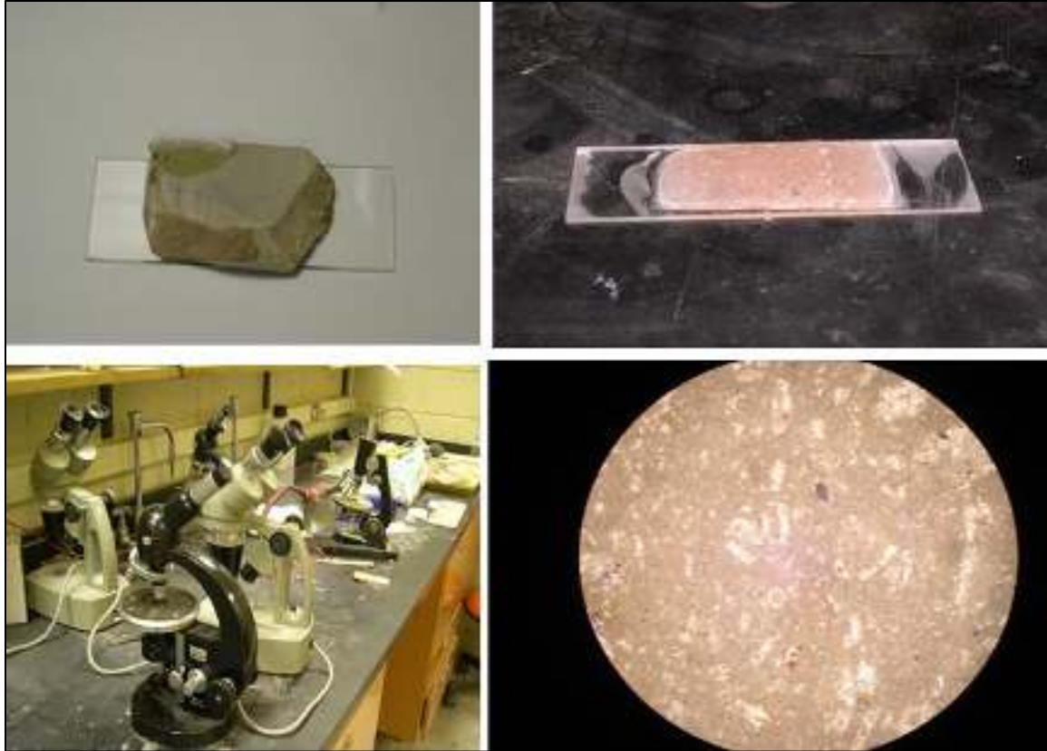
Thin sections prepared in rock cutting lab ready for examination in the petrographic laboratory
