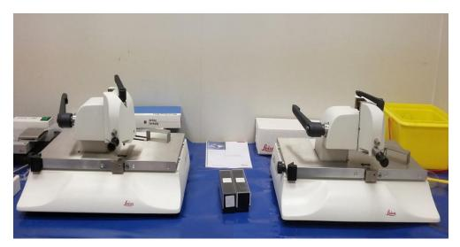
Application: The glass knife maker produces 45° glass knives from 6.4 and 8 mm thick glass.
