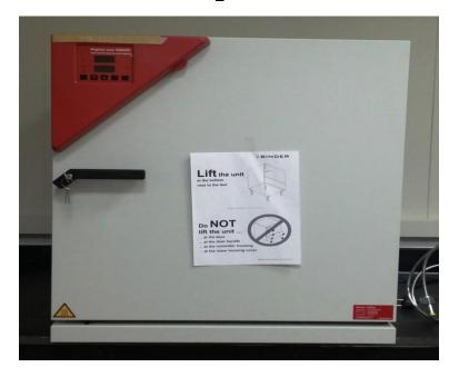
Application: Provides an optimal growth condition for mammalian cells with adjustable  $CO_2$  levels.
