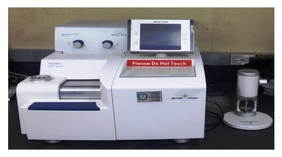
Application: Determination of mass changes on heating (Temp. range 25 to1000°C)
