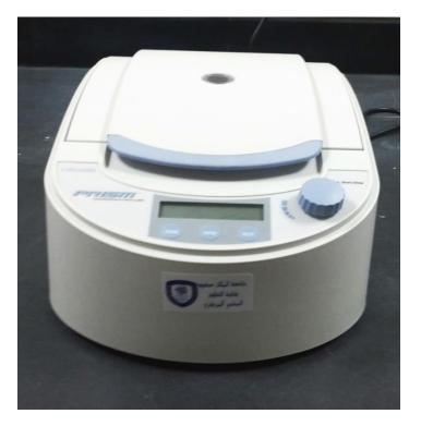
Applications: Centrifuge Eppendorf tubes to a maximum of 15000 RPM
