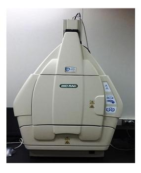
**Application:** The ChemiDoc MP system is an instrument for gel or western blot imaging. It is designed to address fluorescent western blotting, chemiluminescence detection, and general gel documentation applications.
