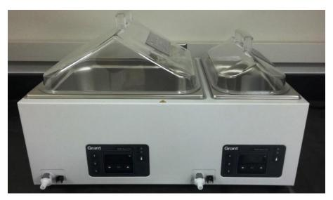
Application: Provides heated water of required temperature, necessary for reactions or experiments requiring specific temperature.
