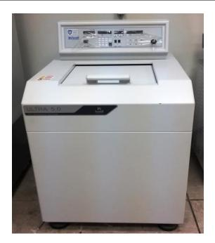
**Application:** Centrifuge with maximum rotating speed: 50,000 rpm (254,345xg) is useful in molecular biology, biochemistry, and polymer science experiments.
