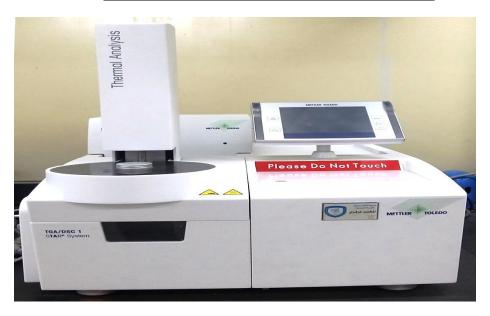
Application: Determination of mass changes on heating (Temp. range 25 to1600°C)
