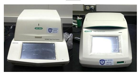
**Application:** PCR reactions and quantitatively measure the amplification of DNA using fluorescent probes.
