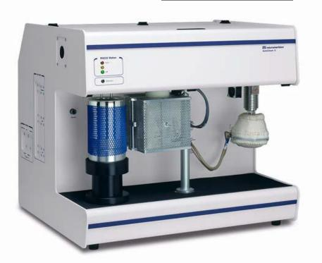
Applications: Temperature-Programmed Desorption, Reduction, Oxidation and Pulse Chemisorptions
