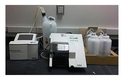
**Application:** Microplate reader instrument is used to detect biological, chemical or physical events of samples in microtiter plates.
