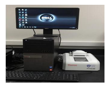
**Application:** Thermo Scientific NanoDrop spectrophotometers is useful to measure the chemicals in small volume of samples around one micro liter within 30 seconds.
