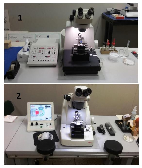
**Application:** This ultramicrotome is designed for cutting ultra-thin sections (<100nm) of sample embedded in resin, using glass or diamond (<u>Diatome, Switzerland</u>) knives.
