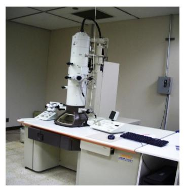
**Application:** The TEM-1011 is a high performance, high contrast, 100 kV TEM with excellent imaging, easy-to-use instrument with an acceleration voltage of 40 to 100 kV. TEM has been used in all areas of biological and biomedical investigations.
