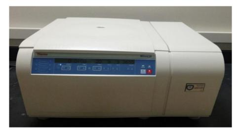
**Applications:** To centrifuge samples in a 15/50 ml falcon tube. Maximum speed that can be attained is 15200 RPM. Also temperature can be set from 4°C to 40°C
