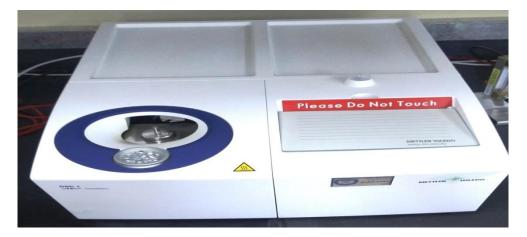
Application: Measurement of glass transition temperature
