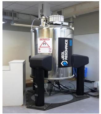
**Applications:** To determine 1D Experiments (1H, 13C, DEPT, NOE), 2D Experiments (COSY, NOESY, HMBC, HMQC, and HSQC), Solid-state NMR (CPMAS, DDMAS)
